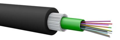
3000N, IND/OUT METAL-FREE CLASS DCA GEL-FILLED, WATER-BLOCKED CENTRAL TUBE CABLE, UP TO 24 FIBRES, GLASS YARN DIELECTRIC ARMOURING AND FIRERES® SHEATH. DIN/VDE: U-DQ(ZN)BH
